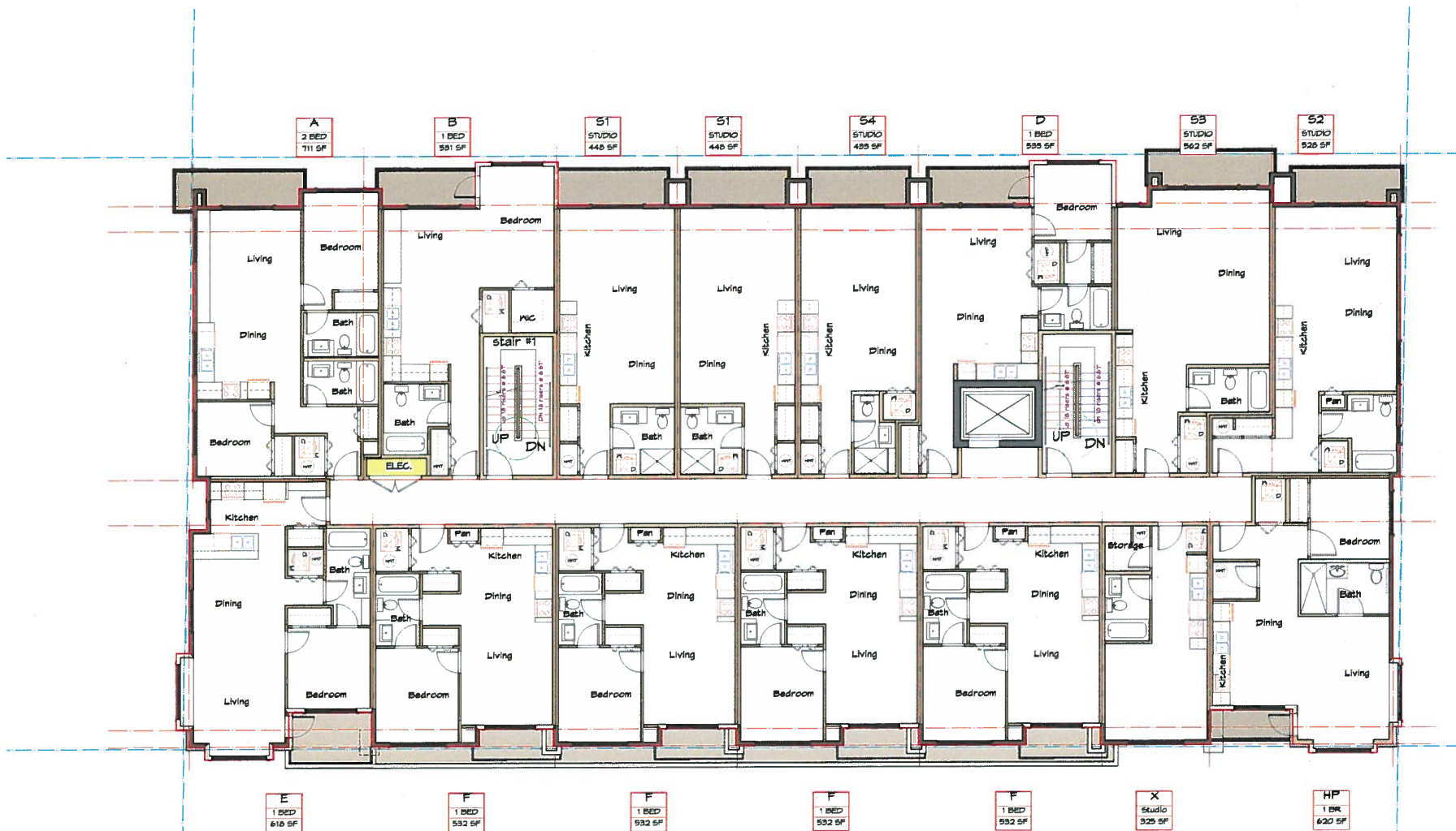
THIRD & FOURTH FLOOR PLAN 3/16"-1'-0" Note: The roof over the townhouses is for the 3rd floor only.
