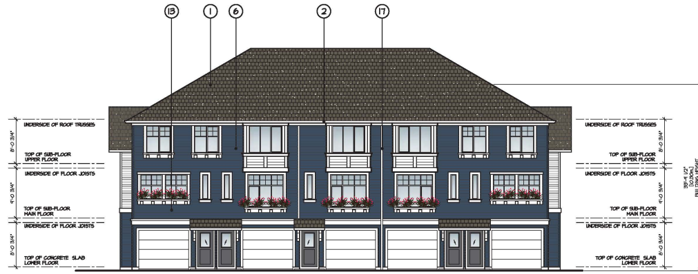
UNIT TYPE 'A4' * UNIT TYPE 'A3' * UNIT TYPE 'M' * UNIT TYPE 'A3' * UNIT TYPE 'A4' FRONT ELEVATION SCALE: 1/8" = 1'-0"
