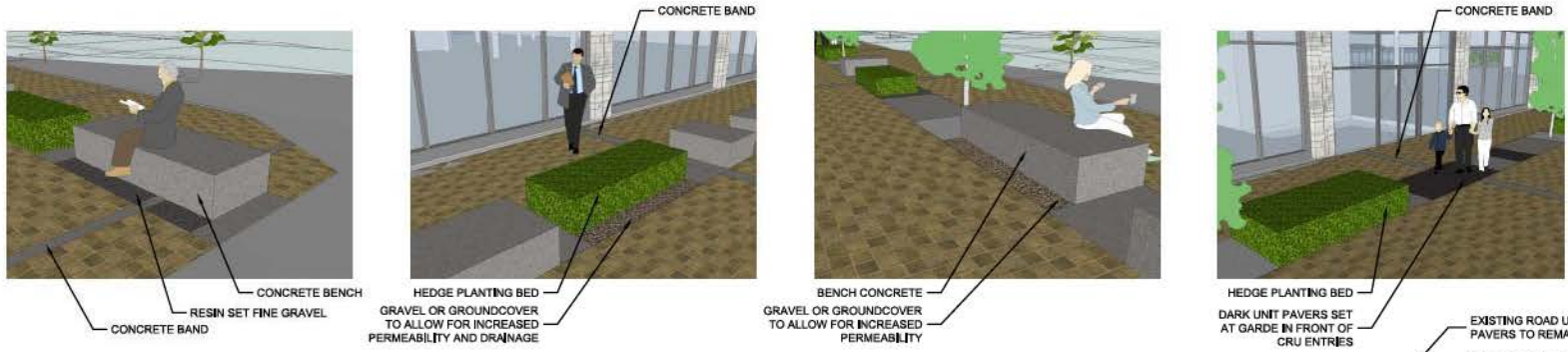
CONCRETE BENCH RESIN SET FINE GRAVEL CONCRETE BAND HEDGE PLANTING BED GRAVEL OR GROUNDCOVER TO ALLOW FOR INCREASED PERMEABILITY AND DRAINAGE BENCH CONCRETE GRAVEL OR GROUNDCOVER TO ALLOW FOR INCREASED PERMEABILITY HEDGE PLANTING BED DARK UNIT PAVERS SET AT GARDE IN FRONT OF CRU ENTRIES CONCRETE BAND
