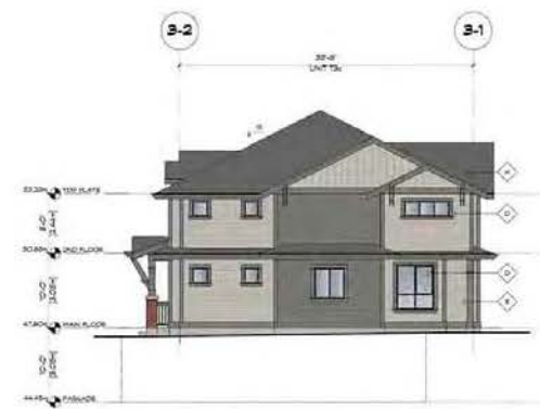
2 BUILDING 3 - SOUTH ELEVATION A2.31 SCALE 1/8"=1'-0"
