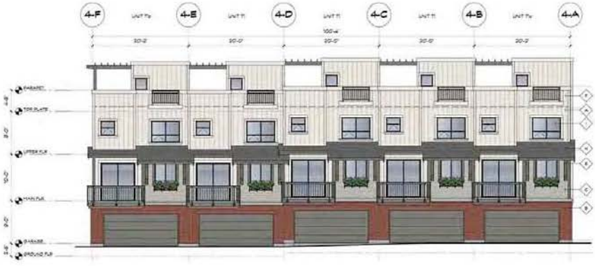
3 BUILDING 4 - REAR ELEVATION A2.41 SCALE 1/8" = 1'-0"
