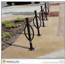
MAGLIN BIKE RACKS MBR970 Series Bicycle Rack; SURFACE MOUNT TO CONCRETE FLOATING SLAB; SLAB TO BE MIN. 18" OUTSIDE EDGE OF SERIES OF RACKS
