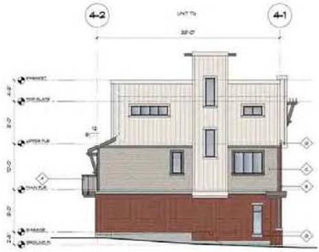
4 BUILDING 4 - SOUTH ELEVATION A2.41 SCALE 1/8" = 1'-0"
