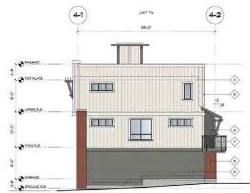
2 BUILDING 4 - NORTH ELEVATION A2.41 SCALE 1/8" = 1'-0"
