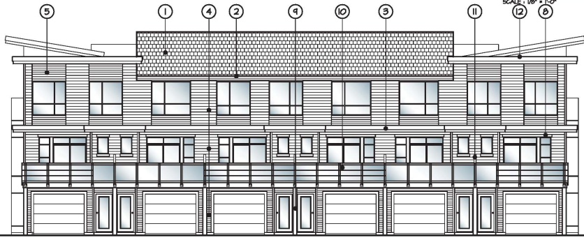
← UNIT 'D6' * UNIT 'D4' * UNIT 'D4' * UNIT 'D5' * UNIT 'D4' * UNIT 'D6' → REAR ELEVATION SCALE: 1/8" = 1'-0"
