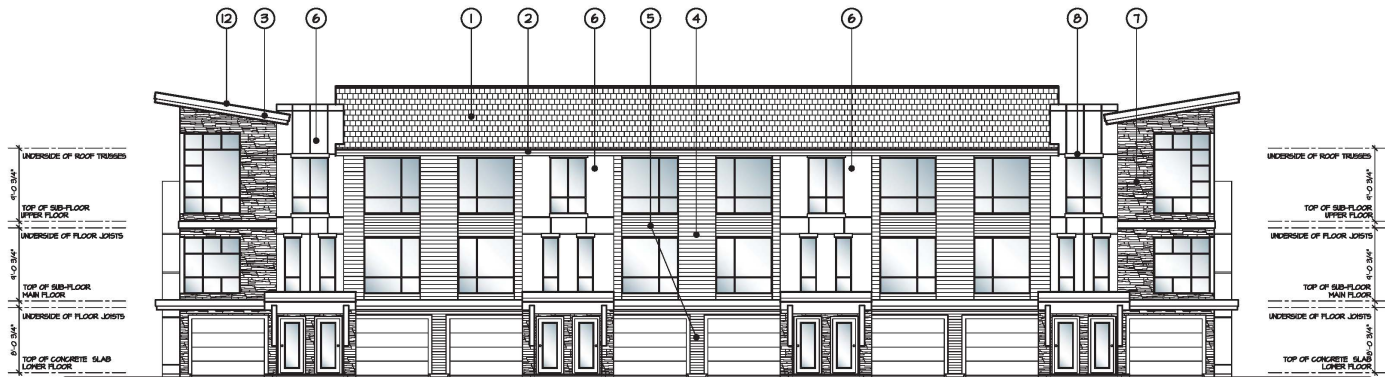
UNIT 'D2' * UNIT 'D' * UNIT 'D' * UNIT 'D' * UNIT 'D' * UNIT 'D' * UNIT 'D' * UNIT 'D2' FRONT ELEVATION SCALE: 1/8" = 1'-0"
