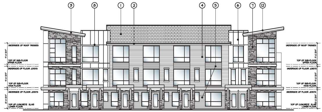
FRONT ELEVATION ← UNIT 'C1' * UNIT 'C2' * UNIT 'C3' * UNIT 'C4' * UNIT 'C5' * UNIT 'B' * UNIT 'A' → SCALE: 1/8" = 1'-0"
