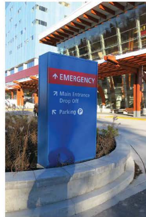
SIGN TYPE 3.0 SECONDARY PYLON Permanent secondary pylon is internally lit with a closed base.
