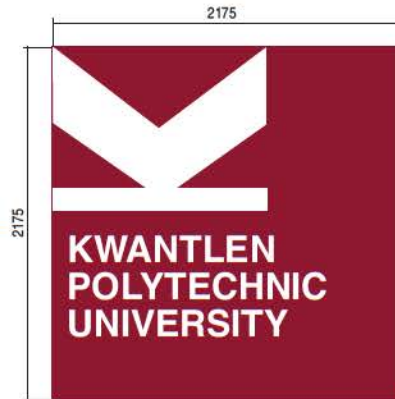
Type N.85: 50± thick x 2175 x 2175mm internally-illuminated (L.E.D.) sign box.
