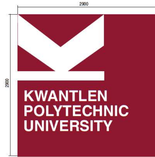
Type N.114: 50± thick x 2900 x 2900mm internally-illuminated (L.E.D.) sign box.
