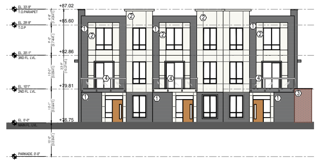
2 BUILDING-1 East Elevation Scale: 1/8"=1'-0"
