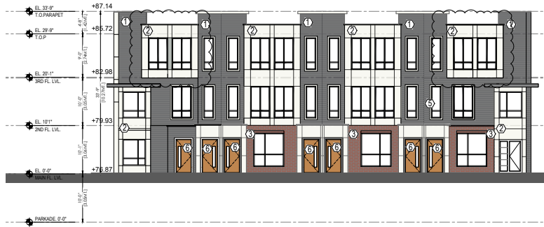
1 BUILDING-2 East Elevation Scale: 1/8"=1'-0"
