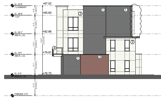
4 BUILDING-1 North Elevation Scale: 1/8"=1'-0"
