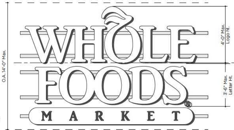
D ANCHOR TENANT FASCIA SIGN - ELEVATION SCALE: 3/8" = 1'-0"
