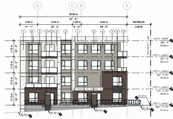
2 EAST ELEVATION (162 STREET) A-301.C 1" = 10'-0"
