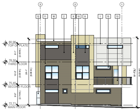
1 BUILDING 7- SOUTH ELEVATION SCALE: 1/16" = 1'-0"
