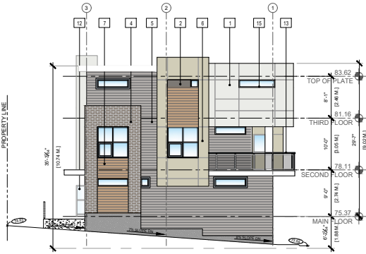
1 BUILDING 10- EAST ELEVATION SCALE: 1/16" = 1'-0"
