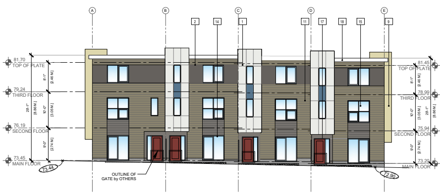
4 BUILDING 6- EAST ELEVATION SCALE: 1/16" = 1'-0"
