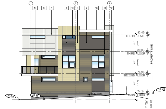
4 BUILDING 8- SOUTH ELEVATION SCALE: 1/16" = 1'-0"
