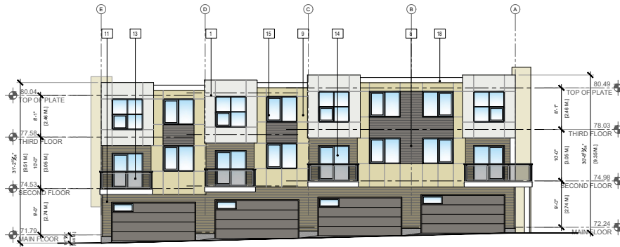
3 BUILDING 3- WEST ELEVATION SCALE: 1/16" = 1'-0"
