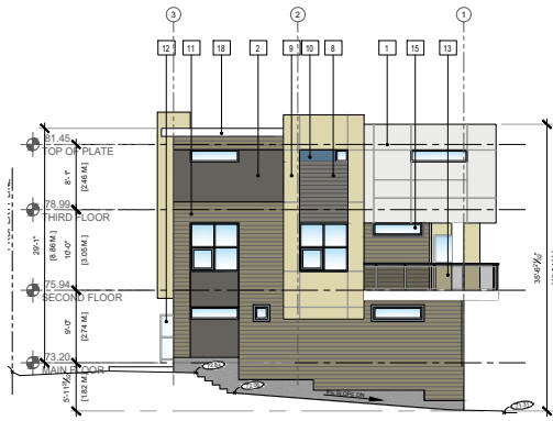
1 BUILDING 6- NORTH ELEVATION SCALE: 1/16" = 1'-0"
