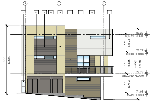
3 BUILDING 4- EAST ELEVATION SCALE: 1/16" = 1'-0"
