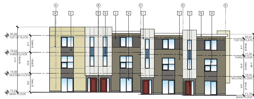
4 BUILDING 3- EAST ELEVATION SCALE: 1/16" = 1'-0"
