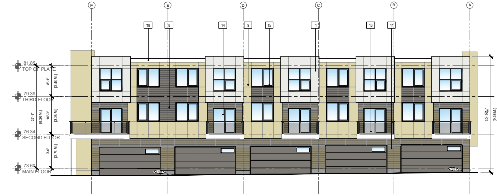
2 BUILDING 9- SOUTH ELEVATION SCALE: 1/16" = 1'-0"
