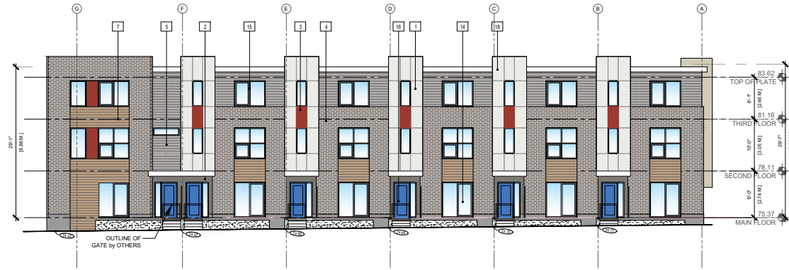
4 BUILDING 10- SOUTH ELEVATION SCALE: 1/16" = 1'-0"
