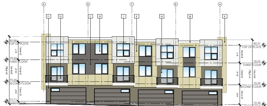
3 BUILDING 7- EAST ELEVATION SCALE: 1/16" = 1'-0"
