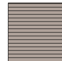
15 EXTERIOR HIGH DENSITY FIBRE CEMENT SIDING TO MATCH ( HARDIE OR SIMILAR) COLOR ( COFFE BEAN BROWN OR SIMILAR)
