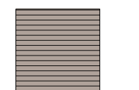
15 EXTERIOR HIGH DENSITY FIBRE CEMENT SIDING TO MATCH ( HARDIE OR SIMILAR) COLOR ( COFFEE BEAN BROWN OR SIMILAR)
