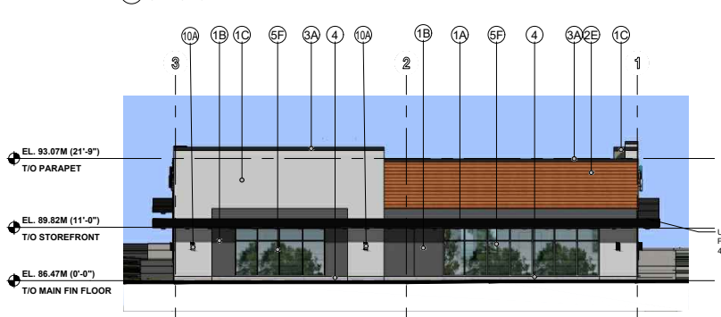
BUILDING B - EAST ELEVATION (132 STREET) SCALE: 1/8" = 1'-0"
