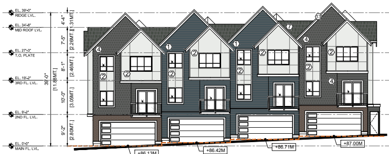
1 Building-7 South Elevation Scale: 1/8"=1'-0"
