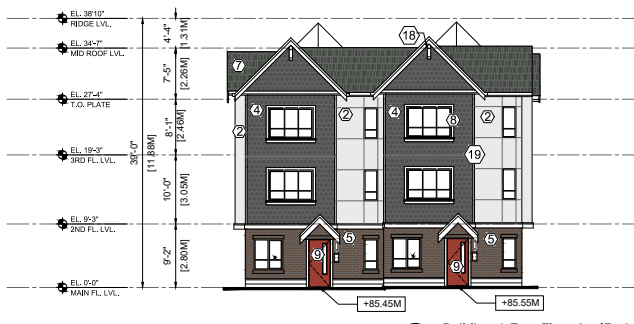
2 Building-1 East Elevation (Facing 165a St) Scale: 1/8"=1'-0"
