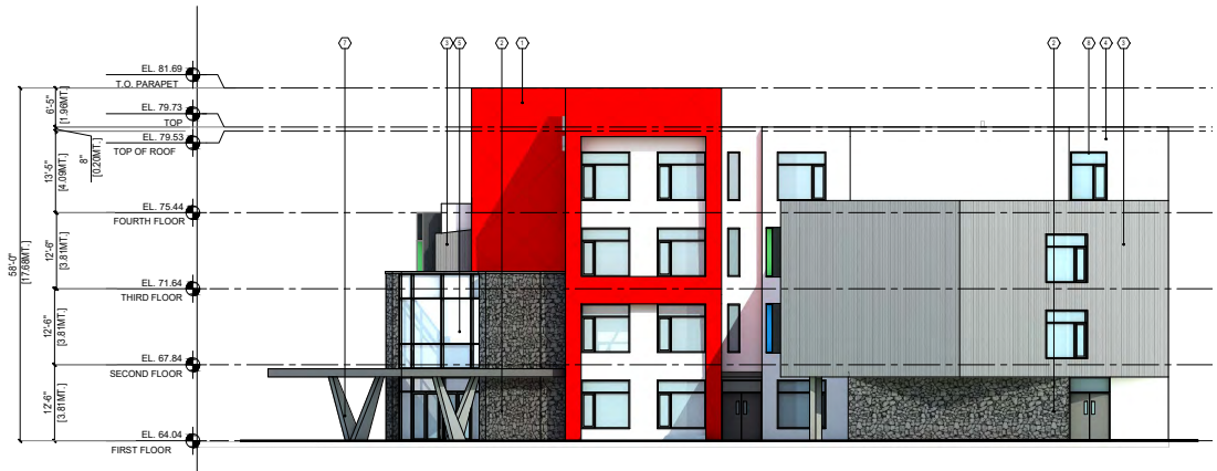
1 SCHOOL- WEST ELEVATION SCALE : 3/32" = 1'-0"
