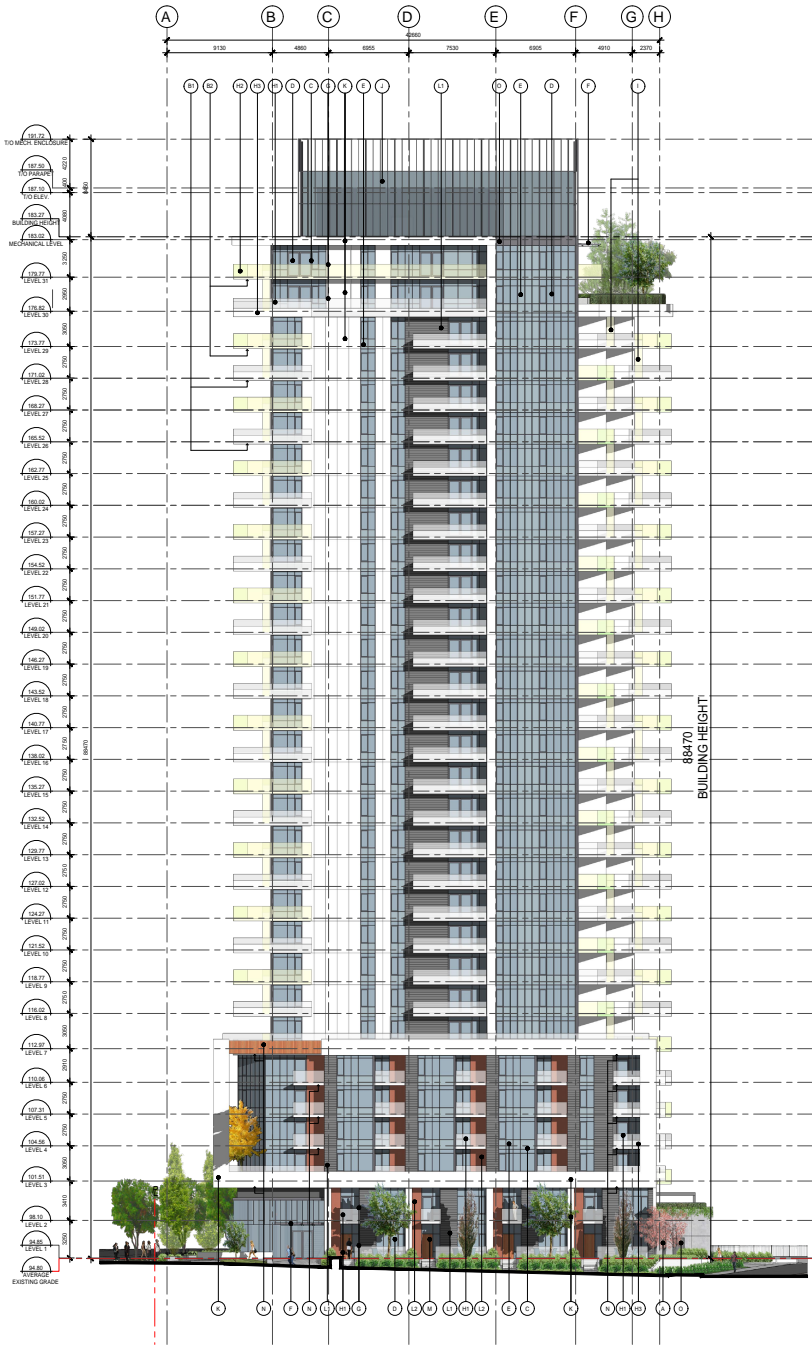
1 BUILDING ELEVATION - WEST 1150
