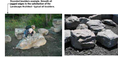
Dimensions of boulders: L (large = 1200mm x 900mm x 600mm) M (medium = 900mm x 600mm x 450mm) S (small = 600mm x 450mm)
