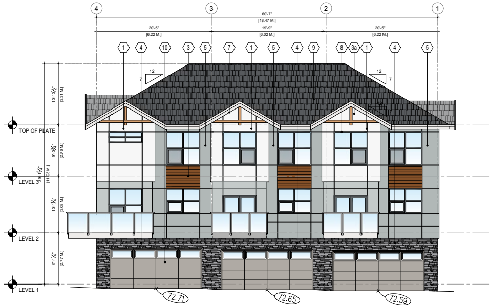
1 BLDG 9 - NORTH ELEVATION SCALE: 3/16" = 1' - 0"
