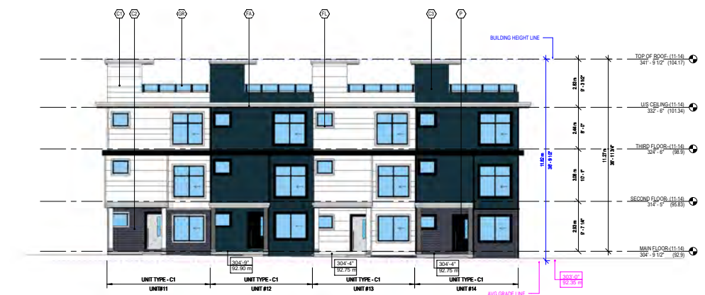
1 NORTH ELEVATION/PEDESTRIAN CORRIDOR DP-6.41 1/8" = 1'-0"
