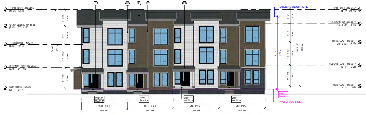
1 SOUTH ELEVATION DP-6.131 1/8" = 1'-0"
