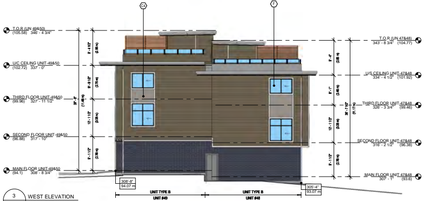
3 WEST ELEVATION DP-6.13 1/8" = 1'-0"
