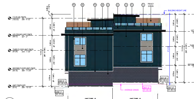
3 WEST ELEVATION DP-6.191 1/8" = 1'-0"
