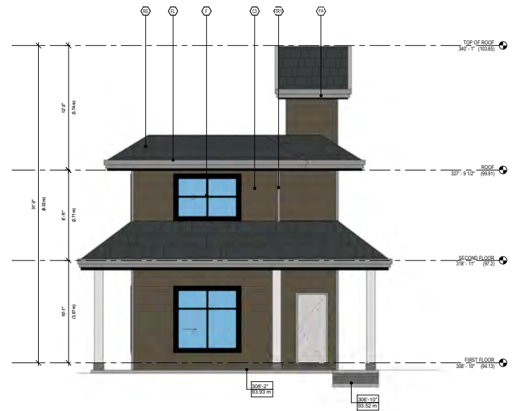
2 SOUTH ELEVATION DP-6.02/ 1/4" = 1'-0"
