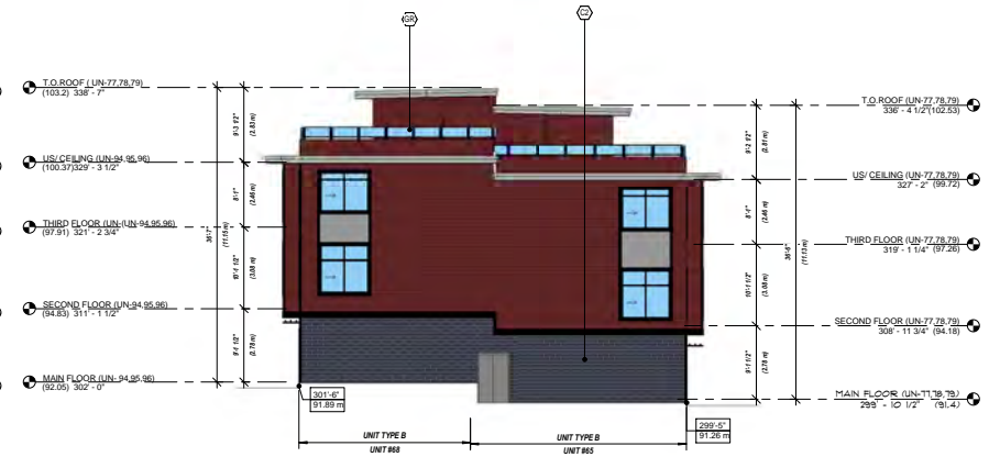
4 WEST ELEVATION DP-6.201 1/8" = 1'-0"
