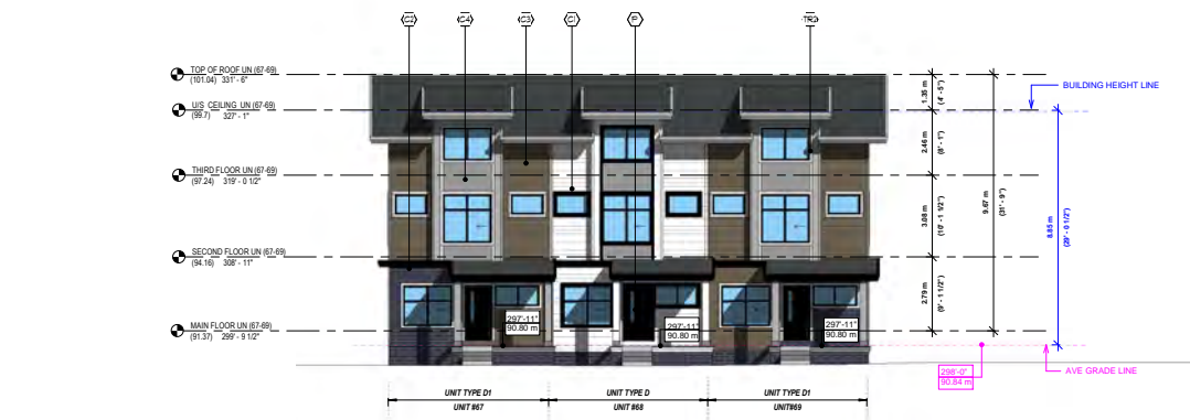
1 SOUTH ELEVATION DP-6.165 1/8" = 1'-0"
