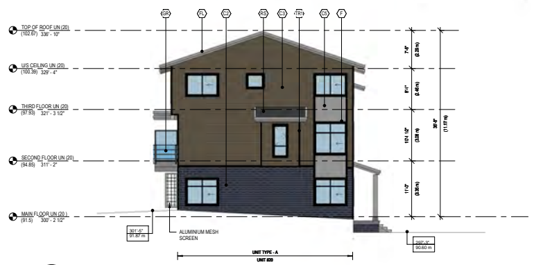
3 NORTH ELEVATION PEDESTRIAN (CORRIDOR) DP-6.61 1/8" = 1'-0"
