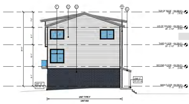
3 WEST ELEVATION BP-6.141 1/8" = 1'-0"
