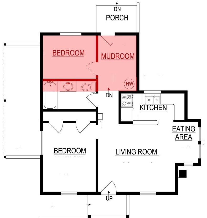
Figure 65: Cottage plan with addition in red (drawing by Barnett Dembek Architects Inc.)
