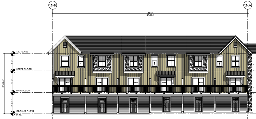
3 BUILDING 12 - ELEVATION SOUTH Scale: 1/100
