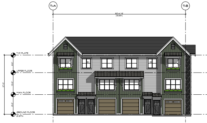
1 BUILDING 11 - ELEVATION NORTH Scale: 1/100
