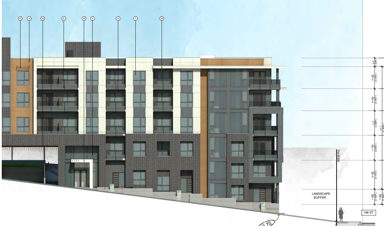
2 SOUTH ELEVATION ALONG 196 AVE. (BLDG#1) PART-B 3/32" = 1'-0"
