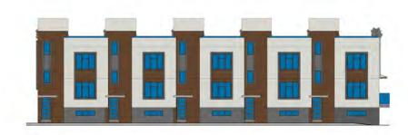
3 Typology 1 - 6 Unit Block - North Elevation 1:100
