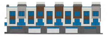
1: 100 Typology 1 - 6 Unit Block - South Elevation
