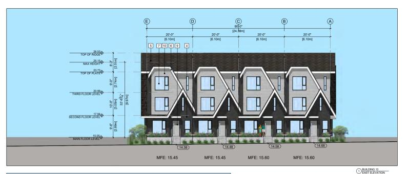
(1) (2) 32'-6" [9.91m] 4 2 4 7 5 11 TOP OF RIDGE 25.15 MAX HEIGHT TOP OF PLATE THIRD FLOOR LEVEL SECOND FLOOR LEVEL п MAIN FLOOR LEVEL (15.50) 14.68 MFE: 15.60 2 BUILDING 13 NORTH ELEVATION
