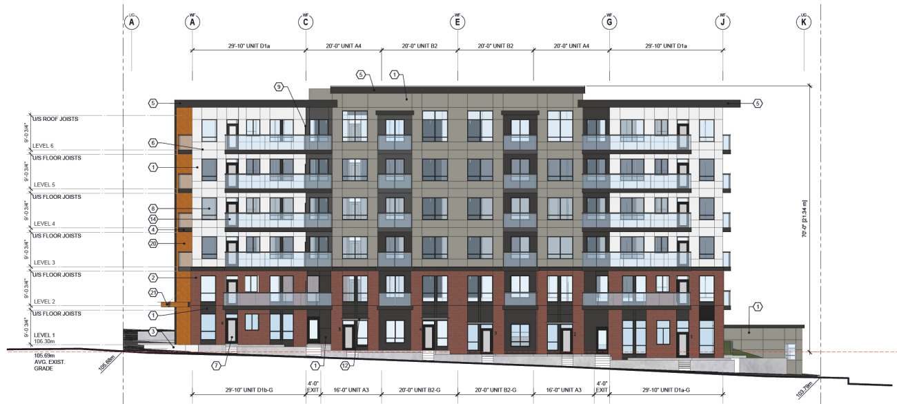
SOUTH ELEVATION (104 AVENUE) SCALE: 3/32" = 1'-0"
